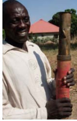
Fig. 11 Damaged Cylinder Brass lining.
