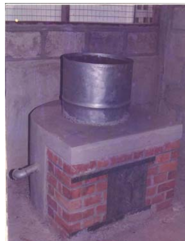
An appropriate furnace built with Bricks and fitted with out-let drain to die and de-
